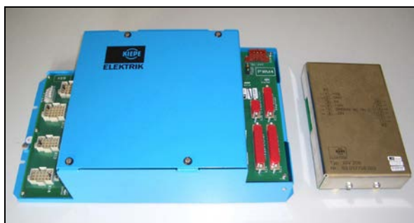
Supervisory Control Unit – central control element
